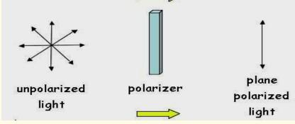
If the vibration are along a line in a plane perpendicular to the direction of propagation of light. The light is called plane polarised or the linearly polarised light.
